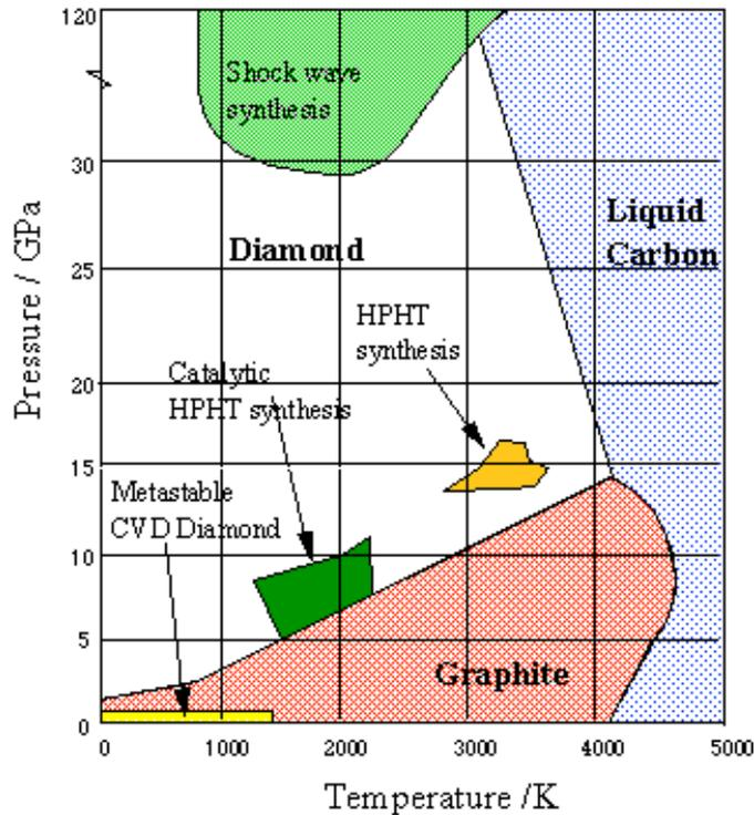
**Figure 1.** The phase diagram for diamond and graphite, depicting the pressure-temperature regions that correspond to the liquid and the two solid states of the element carbon. Note that the solid form known as diamond sits above the solid form known as graphite on the pressure scale. Inset regions identify where various man-made processes lie. From Bundy (1980)
